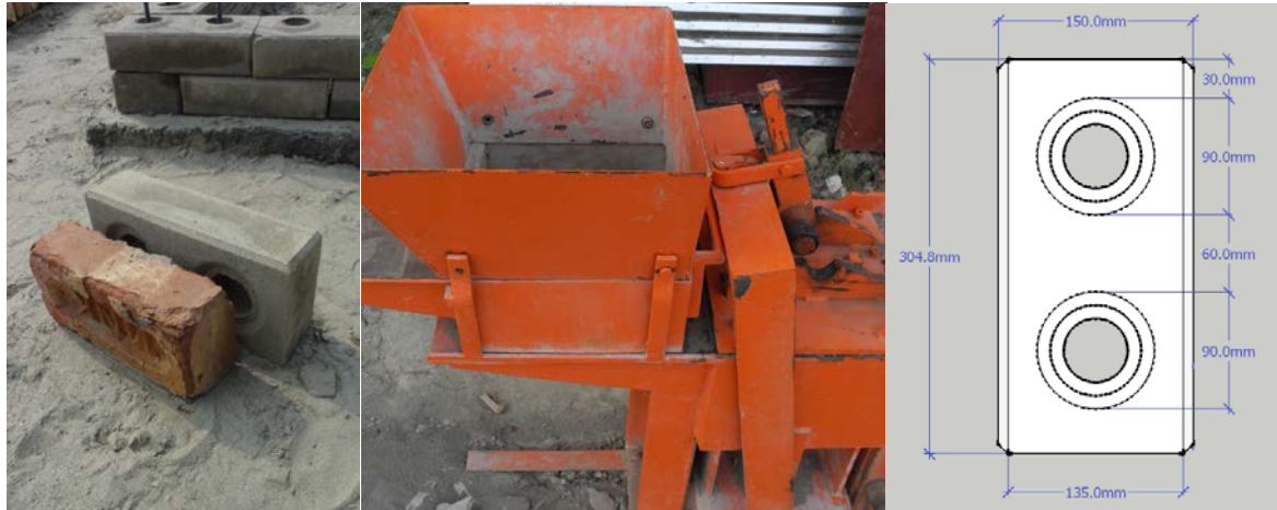
Figure 2: Brick Machine is used to produce CEB which are 1.5 times bigger than regular bricks.
