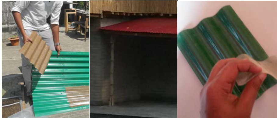
Figure 3: Jute Composite Tin (JCT) made from jute, resin and crystalizing agents.
